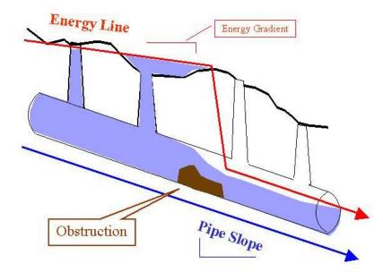
upstream. And the slope of the energy line can <u>also</u> be gentler than the pipe slope if an overflow is occurring downstream. In fact, scattergraphs of real sewers show them constantly storing and releasing flow, dynamically changing their energy gradient in continuous response to changes in loading; and scattergraphs from real sewers bear witness to developing and active overflows.
