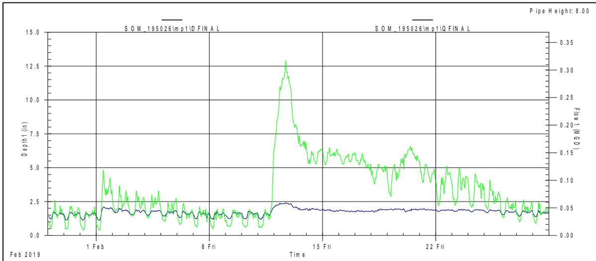
**Graph 6: minor change in level (blue) versus a significant change in flow (green)**
