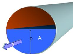
Those engaged in collection system flow measurement rely on A/V or *flow monitors* to conduct their work. Even small collection systems can have thousands of pipe segments and manholes. It would be more favorable to have numerous flow monitors distributed throughout the collection system, but it may be cost prohibitive. Thus, concurrent measurement of many sites can be budget limited.
