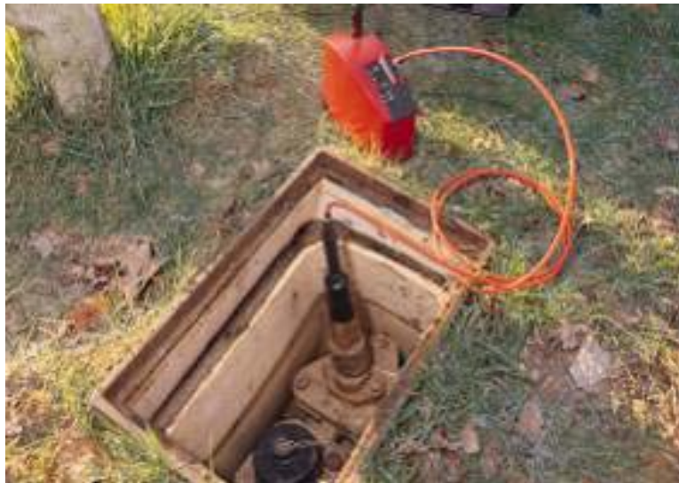
Accelerometer attached to valve body
