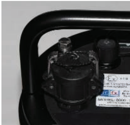
SIM card enclosure with plastic tie
