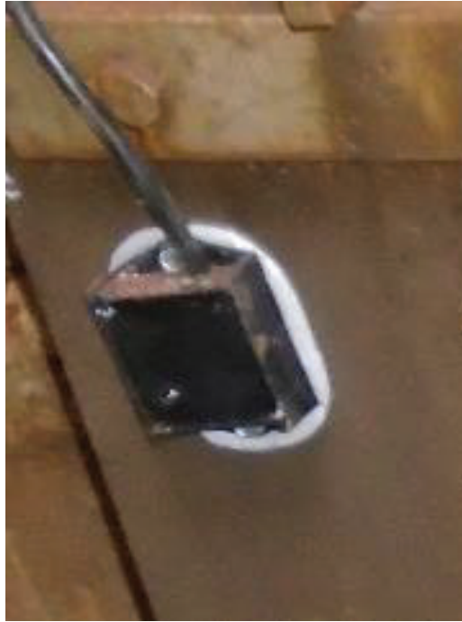
Inclinometer attached using Construction Adhesive
