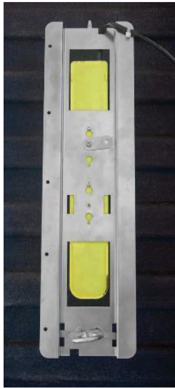
Attach ParaDepth/ParaFlow Sensor to Sensor Bracket
