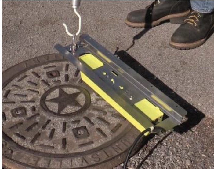
Sensor Bracket Securely Looped on Pole Hook
