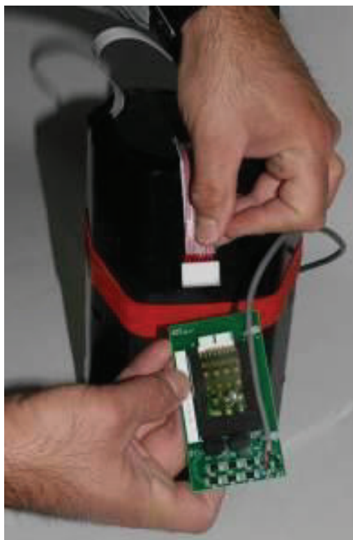
Disconnecting the PCB from the battery pack
