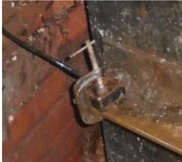
Inclinometer attached using a Stainless Steel Clamp
