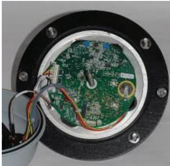
TRITON+ top with processor board attached
