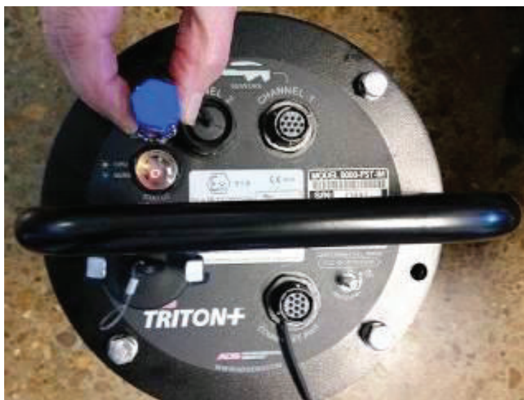
Proper Location for Magnet on Monitor Top
