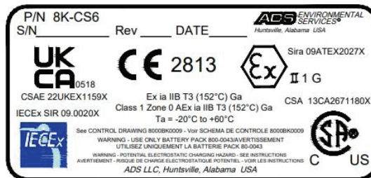
Long Range Depth (CS6) ATEX, IECEX, CSA, UKCA Certification Label
