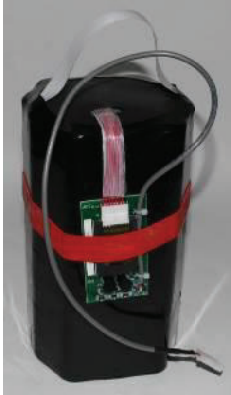
12-volt battery pack without retainer plug
