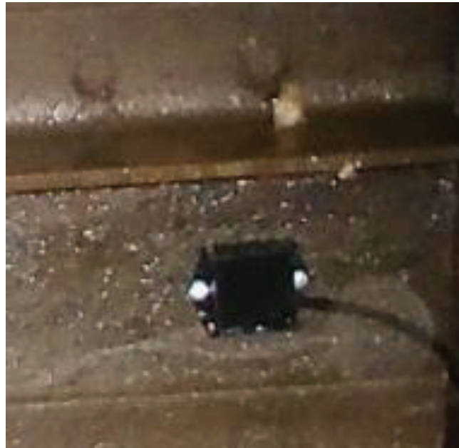
Inclinometer attached using Stainless Steel Screws
