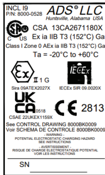
Inclinometer ATEX, IECEX, CSA, UKCA Certification Label
