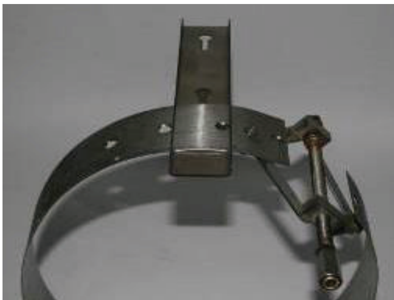
Properly attached spreader mechanism (with Ultrasonic Depth Sensor mounting plate on ring, configured for a Surface Combo)
