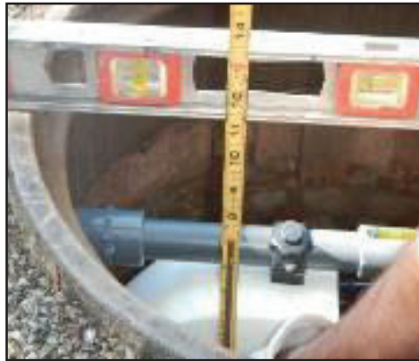
Recording physical offset at measurement intersection
