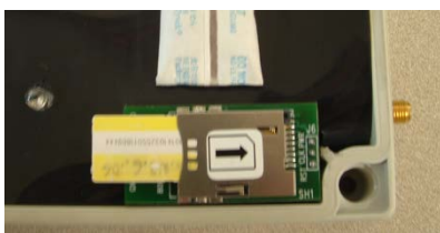
Inserting SIM card into the holder
