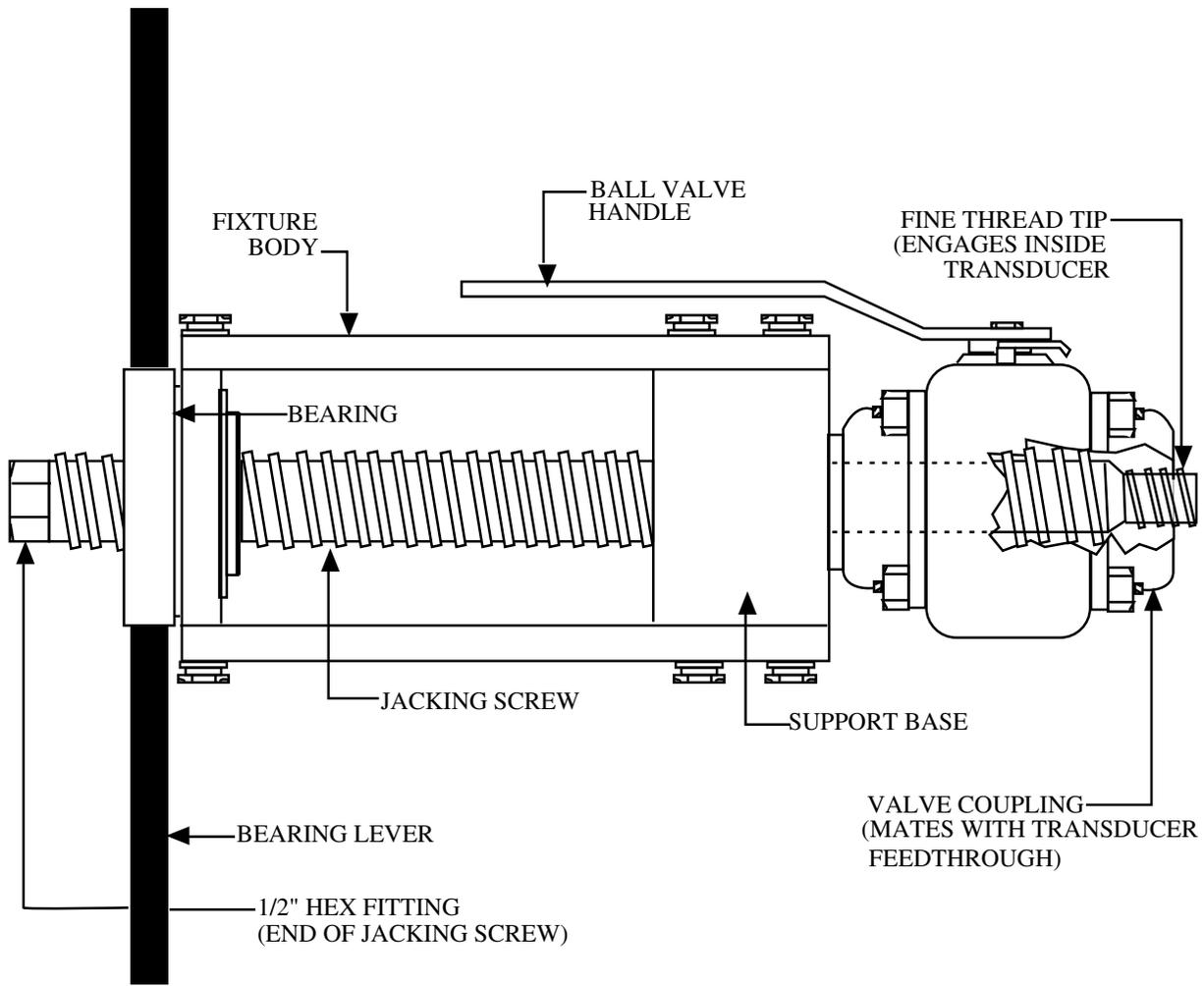
Figure 10-2 7601 Transducer Extraction Tool (uninstalled)
