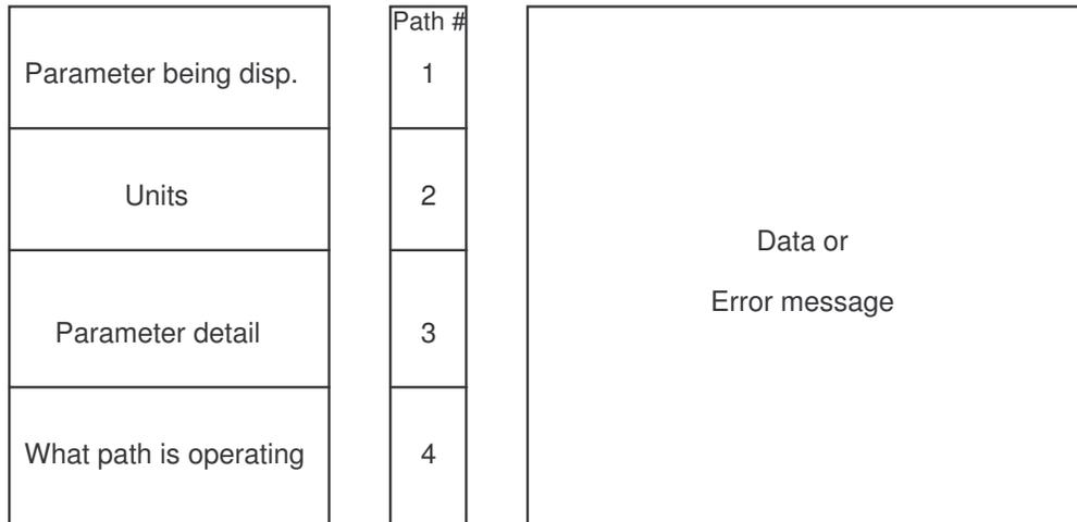
Variables are displayed only when the flowmeter is in “Measure” mode. Immediately after power up, the flowmeter will enter the “Measure” mode, and display whichever display had been selected when the flowmeter was last put into “Measure” mode..
