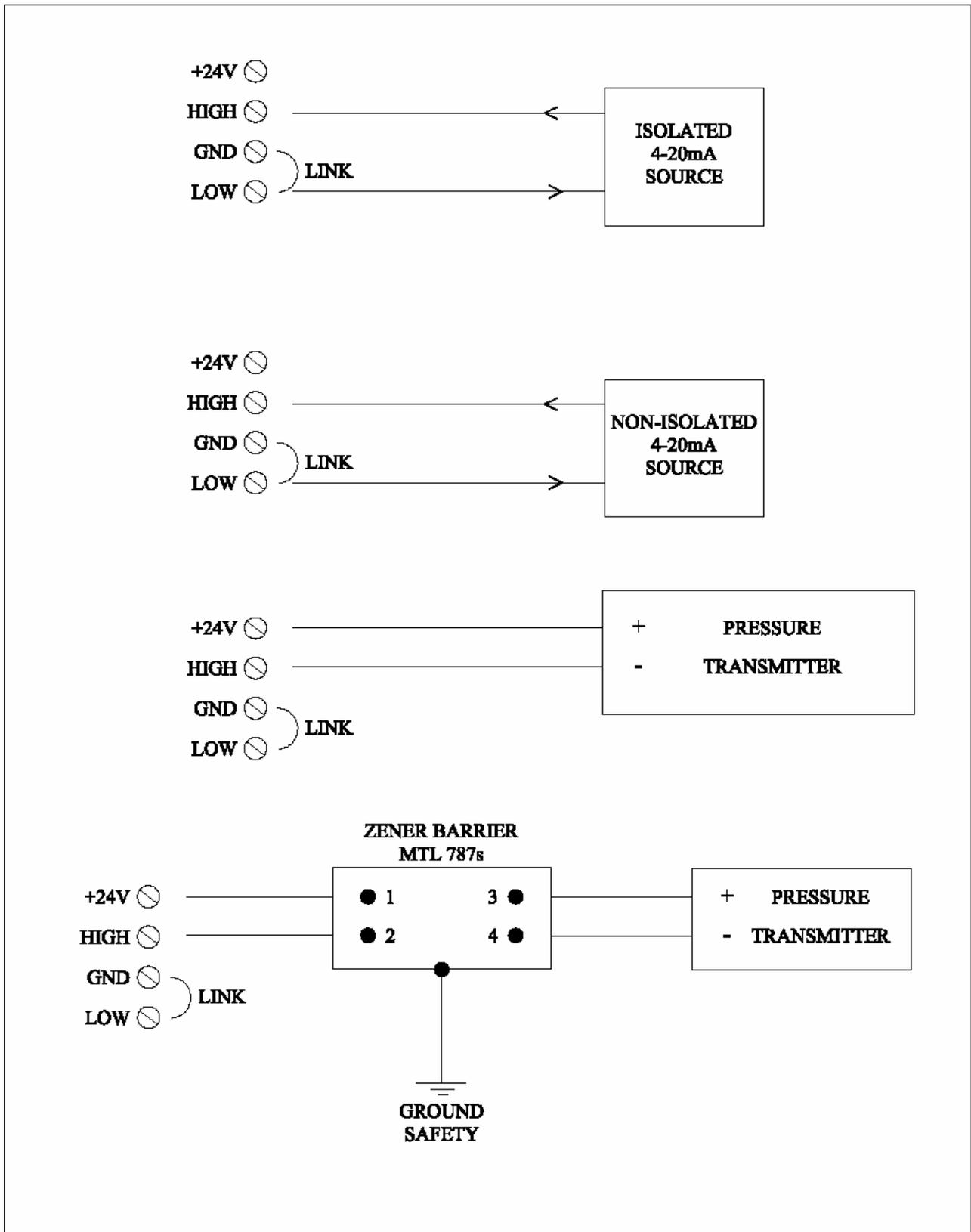
Figure 4-5 Typical Analog Level Connection
