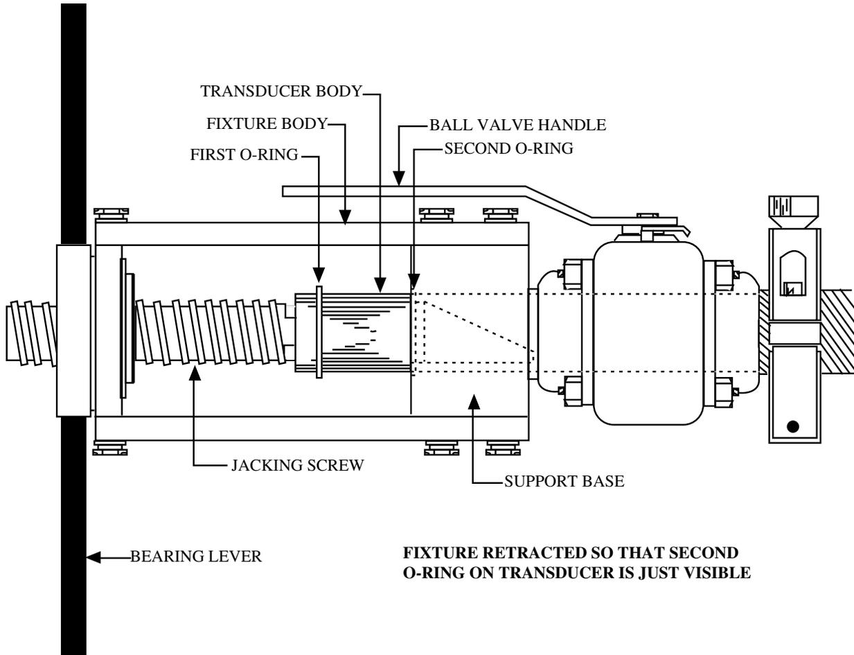
**Figure 10-4 Extracting 7601 Transducer using Withdrawal Tool**
