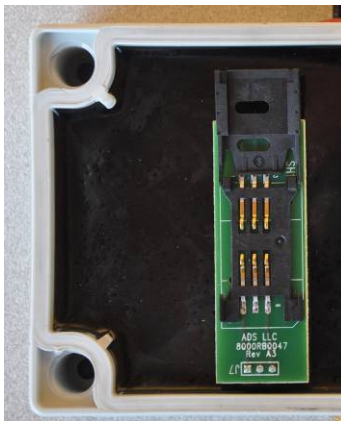
Swinging up hinged clip and inserting card; notice beveled edged of card
