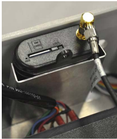
SIM card seated in the EMU modem
