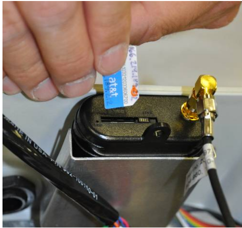
Inserting the SIM card into the EMU modem
