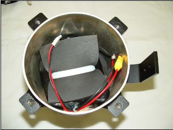
Battery pack seated in monitor (lift out using white strap)
