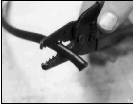
Stripping the external insulation from the telephone cable
