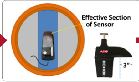
3.5 Ensure Installation of the ECHO Places the Effective Section of the Sensor Directly Over the Channel
