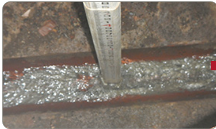
1.1 Measure Distance from the Bottom of the Invert ...
