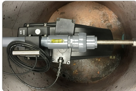
Option 2. Antenna on top of ECHO , Logo Facing Up
