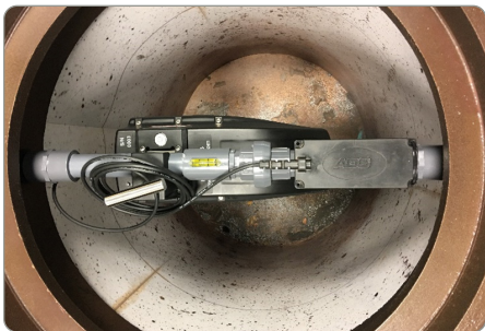
Option 1. Antenna Cabled Tied to Bar, Logo Facing Up
