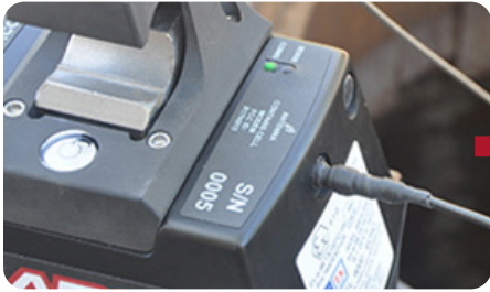
3.1 Attach Antenna to ECHO and Wrap Connection with Rubber Splicing Tape
