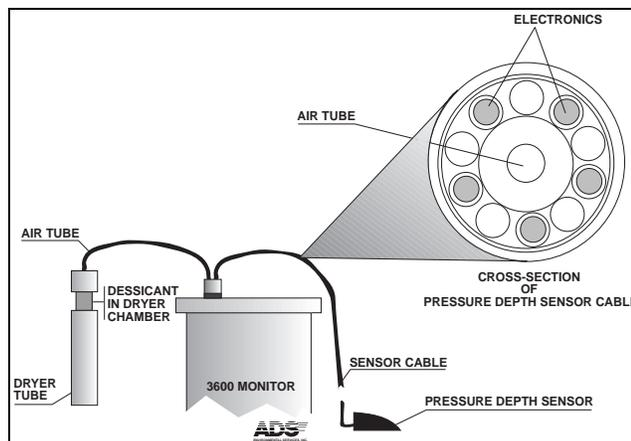
Dryer Tube and Air Tube as Incorporated into the Pressure Depth Sensor Cable
