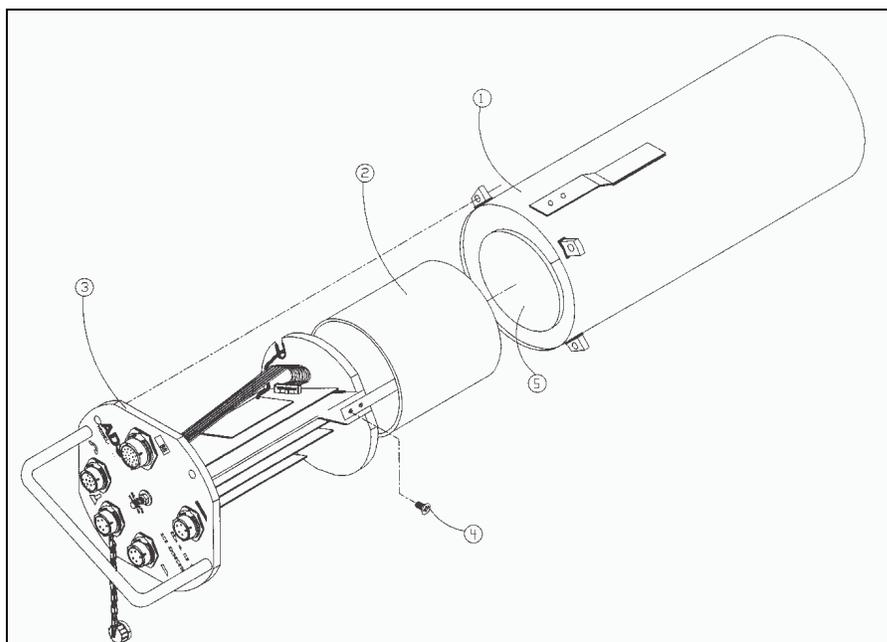
Assembly of the QS3600 IS Flow Monitor
