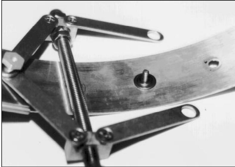
Inserting Washers onto the Spreader Mechanism Screw
