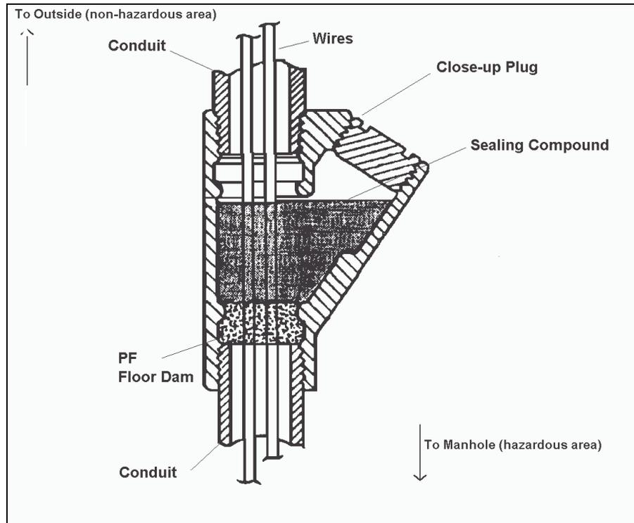
Killark Series EY Sealing Fittings: Relationship between the Conduit, the Communication Cable, the Sealing Compound, and the Close Up Plug
