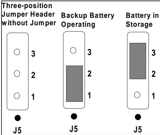
To disable the backup battery, locate Jumper 5 (a three position jumper header). Move the jumper to cover positions 2 and 3. The battery is now disabled. When the jumper is covering positions 1 and 2, the backup battery is operating.
