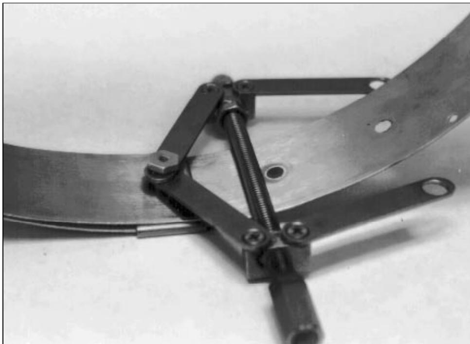
Attaching the Spreader Bars
