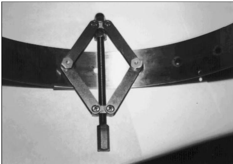
Complete and Attach Spreader Mechanism (Inside Ring View)
