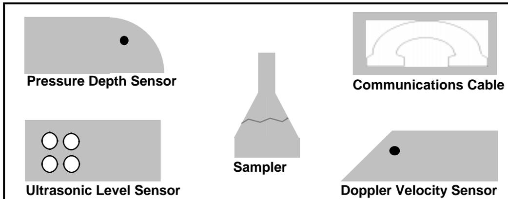
Icons on the Monitor Lid Indicate Proper Cable Connections for Each Port
