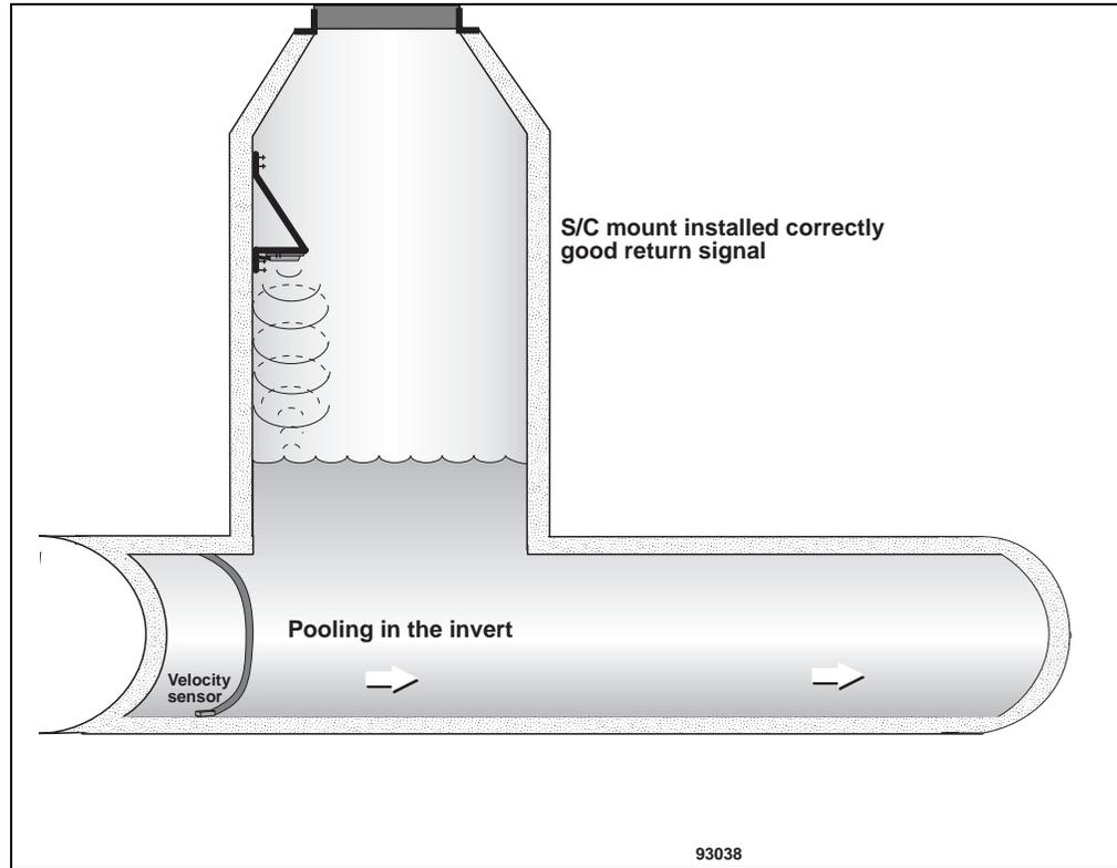
Because the Bracket Mounts onto the Manhole Wall, Be Aware that Rungs and Brick Outcroppings May Affect the Ultrasonic Sensor Readings.
