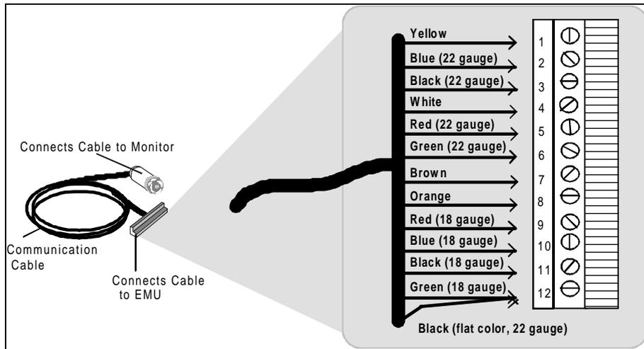
Proper Communication Cable Wire Connections
