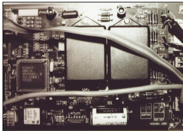
IS Modem on the Processor Board
