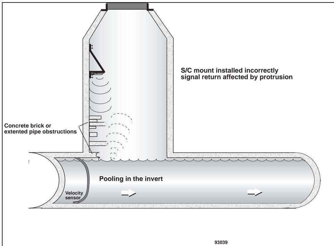
In Some Instances, the **Pulse Command** and **Spare 2** Must Be Adjusted to Record the Correct Depth Readings.
