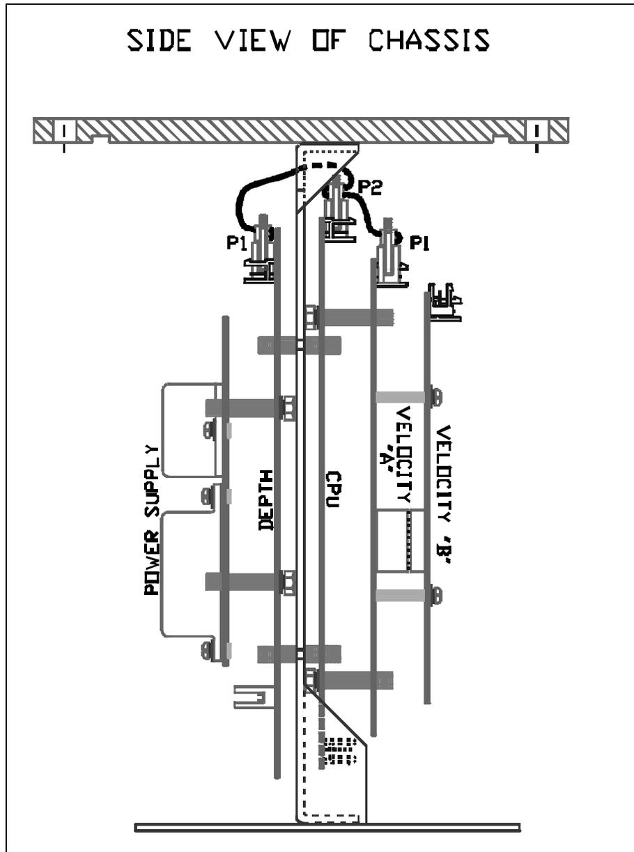
Side View of Flow Monitor Chassis and Assembly
