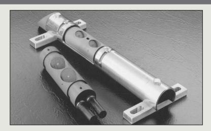
The Accusonic Models 7630 and 7634 are dual-element, internal-mount transducers designed for installation inside buried or encased pipes. The cables from the transducers are brought through a conduit to a penetration assembly which can be located in a small area of exposed pipe.
