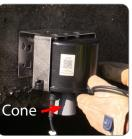
**4.3** Insert the device into the bracket. Place unit housing tabs through the two holes on the bracket. Some flexing of the bracket may be required.
