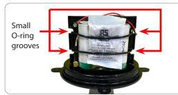
**2.2** Secure the battery and the desiccant to the unit using smallest O-ring, hooking into the 4 grooves (2 on each side). Don't install a damaged or dropped battery.
