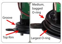
**2.4** Place medium, bagged O-ring in groove of top of unit. Place largest O-ring around top rim of top of unit.
