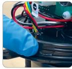
**2.5** Place O-ring grease on both larger O-rings. Proper grease application required for waterproofing and product warranty.
