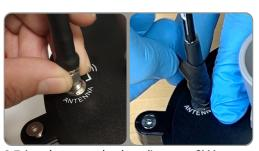
2.7 Attach antenna by threading onto SMA connector. Wrap connection with rubber splicing tape to prevent water intrusion.
