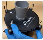
2.6 Press lid assembly into bottom bucket firmly, ensuring O-ring does not squeeze out. Place and tighten screws in a cross pattern.
