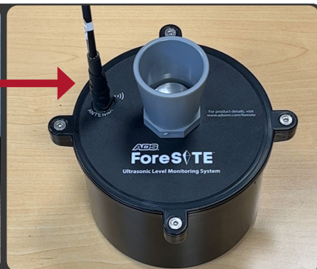
Figure 2 Cover the antenna port and connector using self amalgamating rubber tape.
