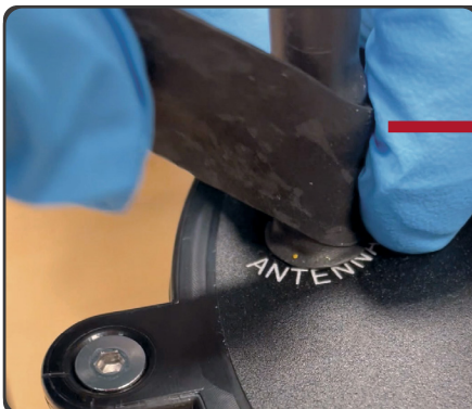
Figure 2 Cover the antenna port and connector using self amalgamating rubber tape.
