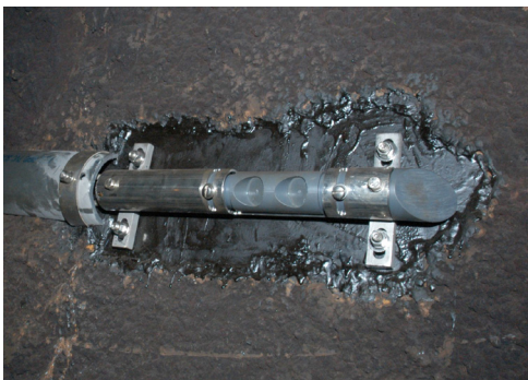
7634 Transducer Mounted in Concrete Pipe
