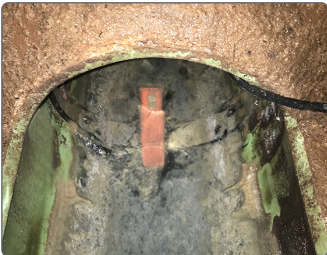
The AV|GATED sensor is built with a rugged Polycarbonate housing that is impact and abrasion-resistant and a contoured form factor that resists debris. The sensor is designed to operate in harsh sewer environments.
