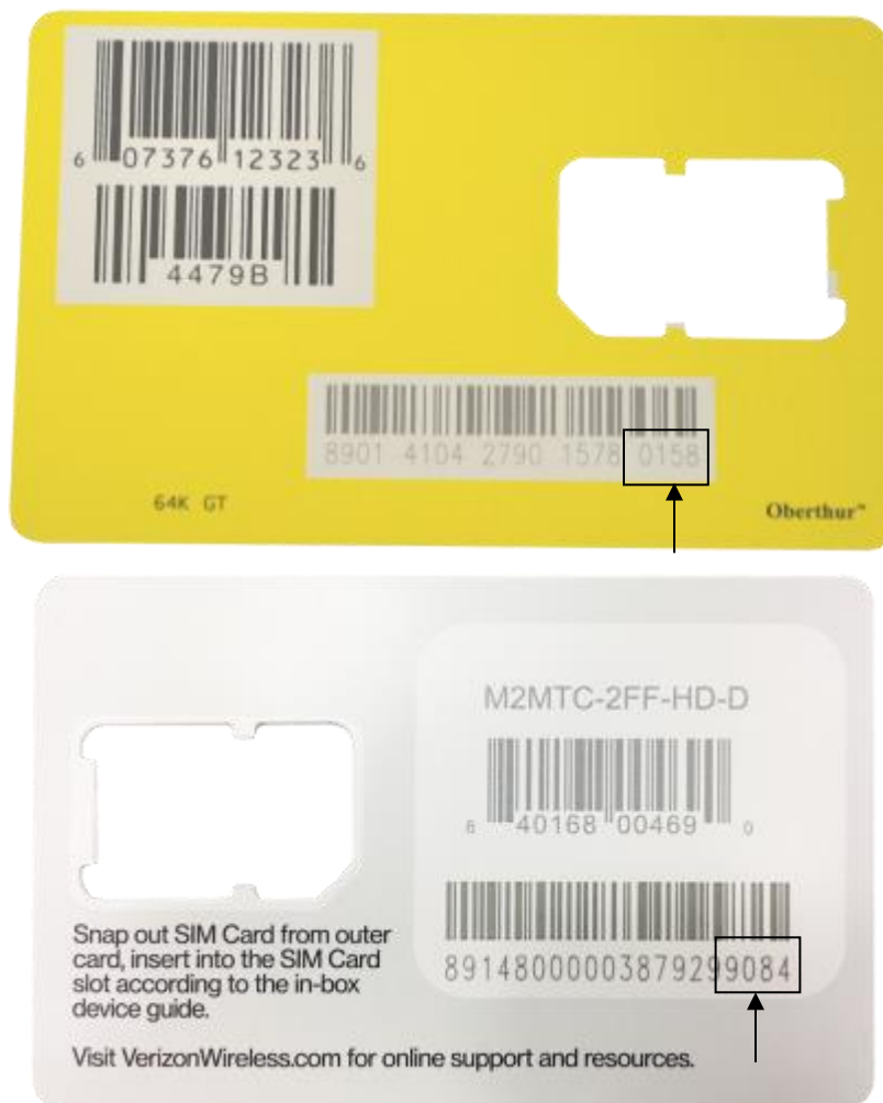
AT&T (top) and Verizon LTE-M (bottom) Punch-out card highlighting last 4 Digits of SIM number
