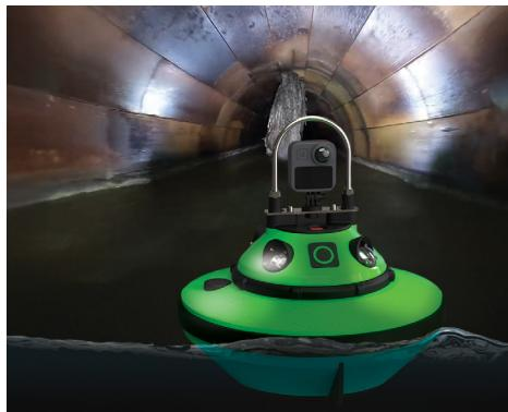
Fortunately, emerging technologies are making proactive sewer monitoring more affordable and accessible. Low-cost, untethered inspection systems such as SewerScout™ from Subterra™ allow municipalities to quickly assess underground pipes without the heavy logistical burden of traditional CCTV inspections.
