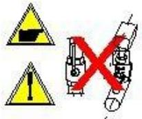
Do not open the ball valve before tightening the two side screws, and affixing the anti-bounce chain
