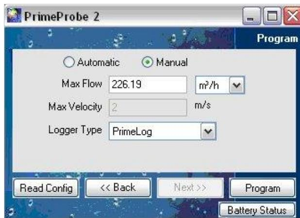
8. Click **Program** to display the FCAL value. This is the value that will be programmed into the connected logger. When using an ADS PrimeLog, make sure the logger is programmed with the sensor type PrimeProbe2 and this FCAL value.
