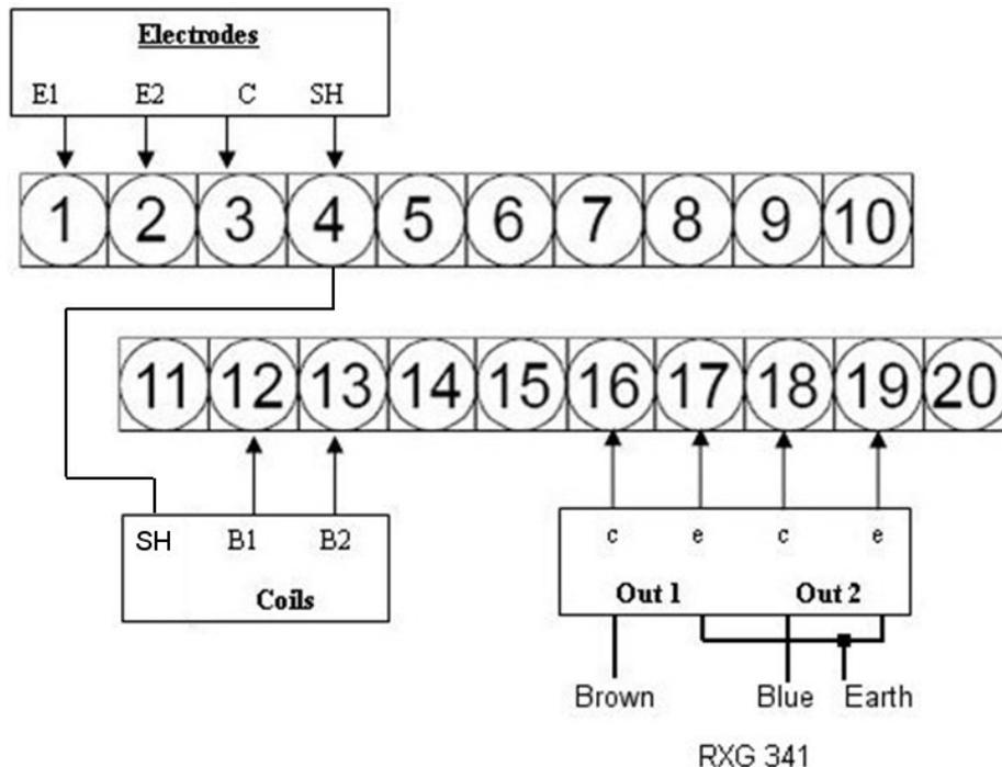
5. To use the pulse output of the PrimeProbe2, connect the appropriate digital output cable to terminals **16 & 17** (*output 1*) and **18 & 19** (*output 2*).
