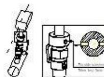
Before opening the ball valve, ensure that the two side screws are tightened, and anti-bounce chain is affixed
