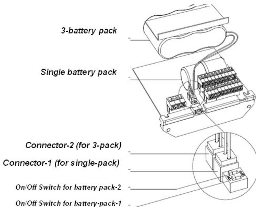
**Note:** With the battery packs connected and the dip switches **ON**, the PrimeProbe2 is now functional. The next step is to configure the converter corresponding to the specific application.
