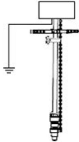
**Note:** Fluctuating flow rates usually are an indication of poor grounding.
