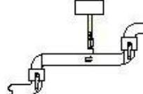
Install PrimeProbe II away from bends or fittings in the pipework
