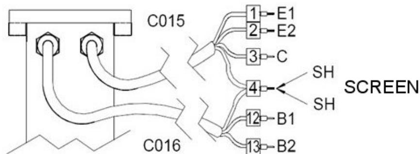
Connect the converter to the sensor in the following way:
