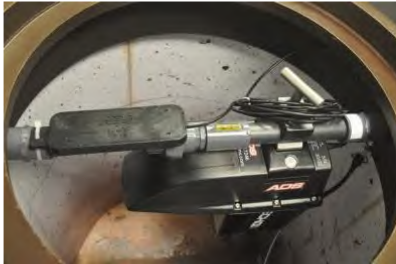
In-manhole antenna installed to mounting bar
