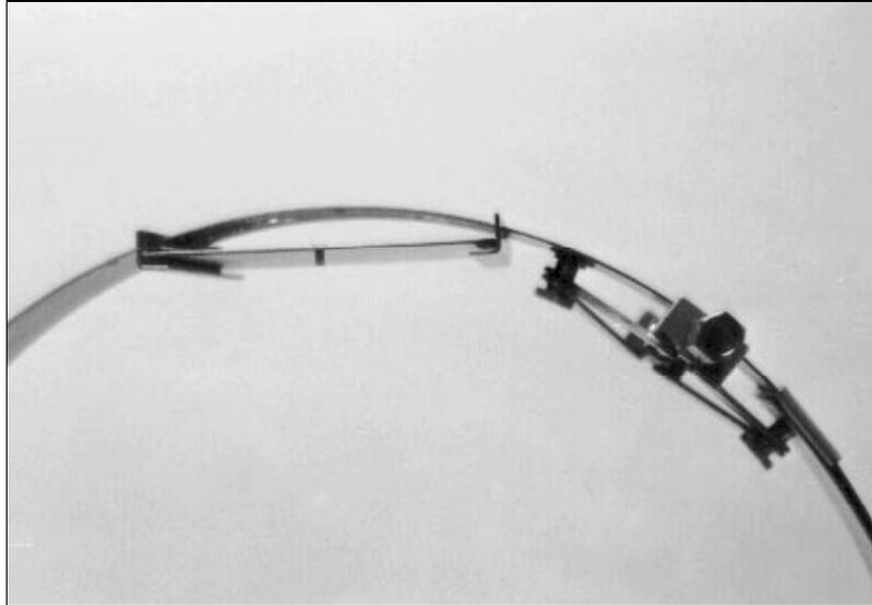
Properly Installed Spreader Mechanism
