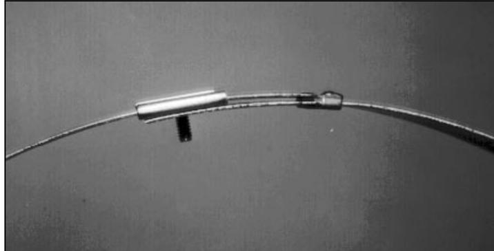
Ring Stabilizer Fully Connected (Side View)
