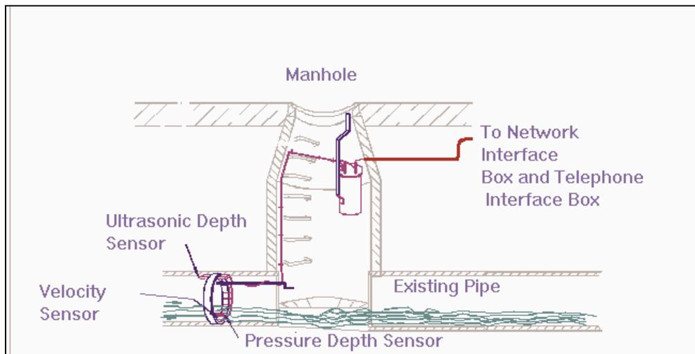
Installed Monitor with an IS Modem
