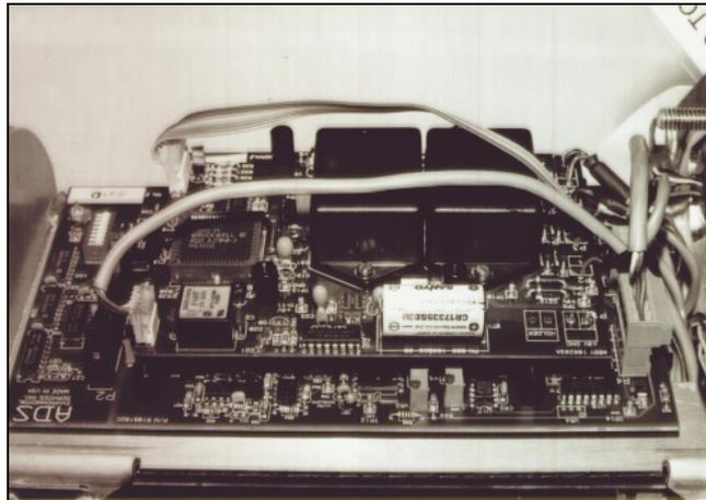
IS Modem on the Processor Board
