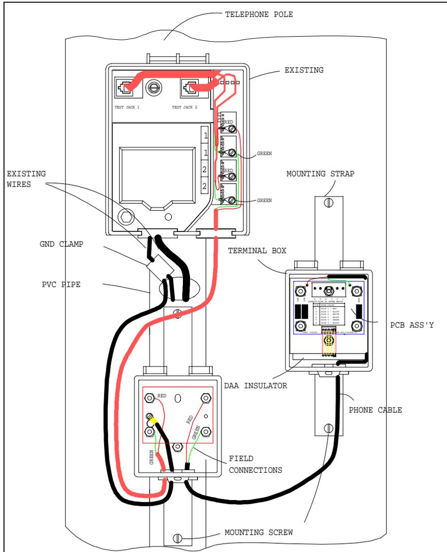
Network Interface Box, Telephone Interface Box, and Lightning Protection Module
