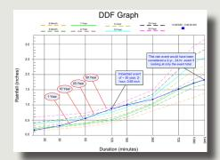
Rainfall Depth-Duration-Frequency analysis shows how a storm behaved and can help explain the cause of overflows.
