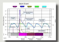
Time series data reveal information about the quantity of flow generated by the system upstream of the monitor.
