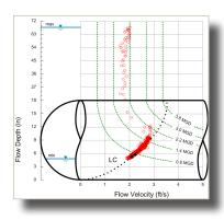
The Scattergraph shown at the left is equipped with iso-Q lines (lines of constant flow rate) and shows that this pipe actually carries 60 percent of its design capacity and is surcharged to a depth of 70 inches. This operational capacity can change over time, and being able to quantify operational capacity is key to spotting "lurking problems."
