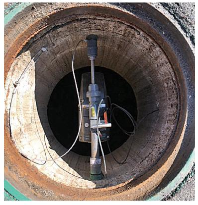
Each remote site has an ECHO ultrasonic monitor that is equipped with the new generation LTE-M communication technology and an all-new antenna. The LTE-M and antenna combination enable installation without any drilling as the antenna is secured to the monitor in the manhole.
