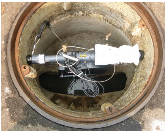
Photograph 2 (top and bottom). Fully stabilized monitors enable high-quality data collection. The units are shown mounted above the invert in each instance. ADS Environmental Services
