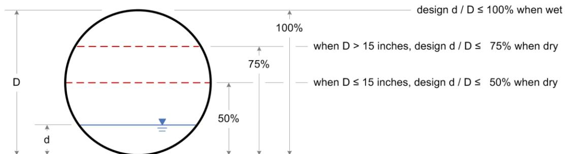
The authors have used such guidelines as KPIs for a number of years to evaluate existing sewer systems under actual operating conditions, and the results can be presented and explored in graphical form as shown in Figure 2. This graphical method evaluates expected maximum hourly average flow depth data within existing sewers in the context of ASCE and WEF sewer design guidance. It can also be adapted to reflect local sewer design requirements, as needed.
