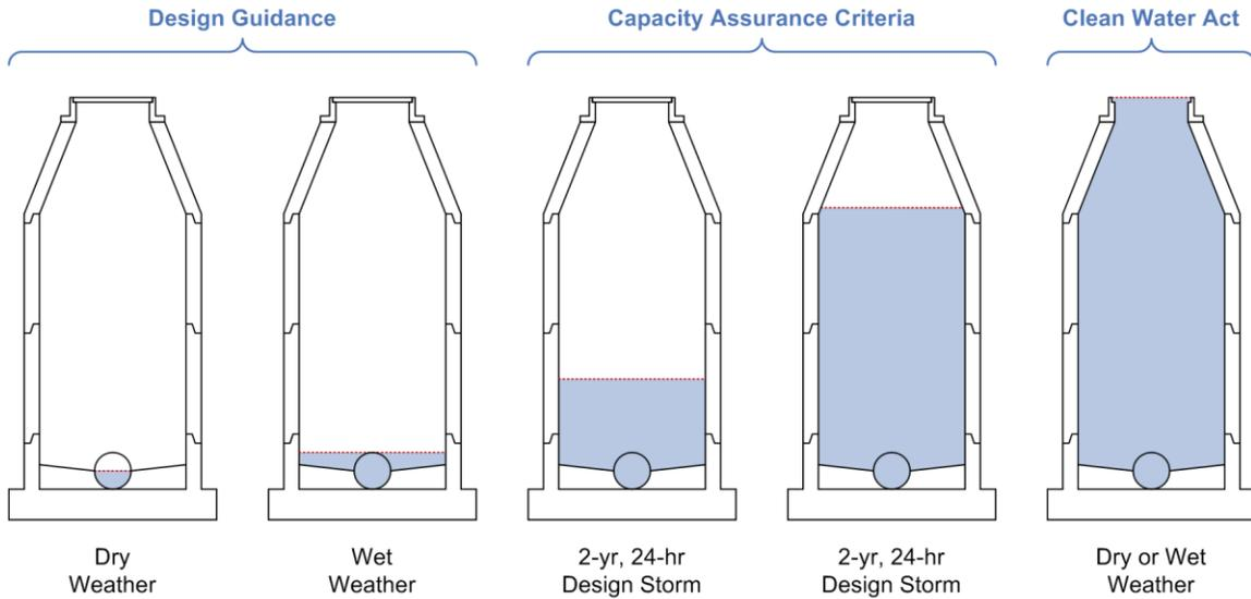
A graphical method to evaluate maximum hourly average flow depth data in the context of both sewer design guidance and capacity assurance criteria is provided in Figure 6. Once again, data from a sewer utility in Tennessee are shown as an example.
